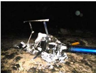
The R44 helicopter involved in that accident, N2153S, experienced a problem on takeoff. The pilot "flew the aircraft all the way to the ground," just as he was supposed to. When the helicopter touched down, it rolled over. As advertised, the two occupants survived the rollover uninjured. But almost immediately, fuel rushed into the cabin, a fire erupted, and both occupants were badly burned.
