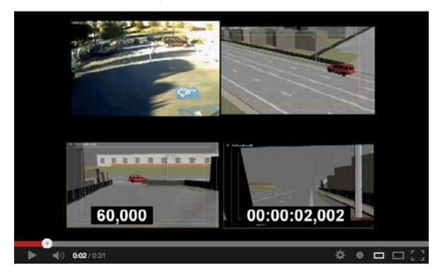
Building on the information above, we also put a virtual camera on the 3D model of the motorcycle to show what the incident would have looked like from that vantage point. This viewpoint demonstrates that the motorcycle driver had no time to react and avoid the collision.
