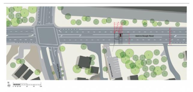
By placing the vehicles in the precise location where they were shown in the actual surveillance video, we could duplicate the speed and movement immediately prior to the incident. We also knew from the police report both vehicles' resting points. With this information, we could then "fill in" the gap of the video to show the movement and impact of the vehicles.
