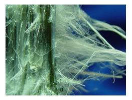
Chrysotile asbestos is the most commonly known type in the Serpentine group and it was the most widely used commercially. Chrysotile asbestos is classified as a sheet silicate, which means it forms flat sheets of long, thin fibers. Chrysotile is more easily woven into cloth than other types of asbestos. (*Pictured: Chrysolite from Asbestorama*)
