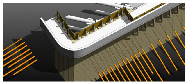
In another example, Mike visualized the entire process of installing the temporary shoring on a project, so that all problems could be identified ahead of time.
