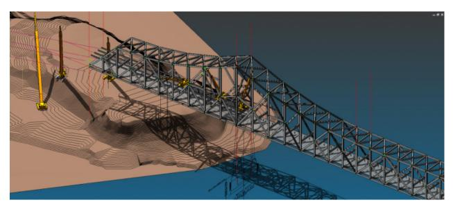
With the 3D modeling capability that is possible now, Mike can create all the models of a crane with the proper length, angles and swings. Therefore, he can determine the lifting capacity at any given location and the exact specifications that will be needed at any point, and see if hazards exist to the workers or the equipment.
