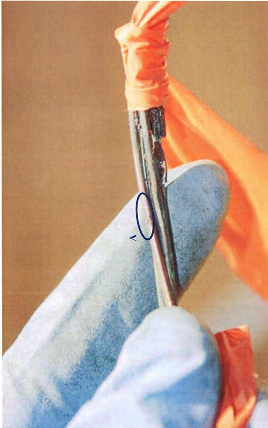
Photograph 13: An oval surrounds apparent electrical activity, as identified during field examination on October 21, 2011, denoted in this supplemental report as region 'A'. This condition presented 22 inches north along the fire alarm circuit conductors (item #5) from the field cut near the ridge (green mark). The artifact developed upslope from and outside of my area of fire origin.
