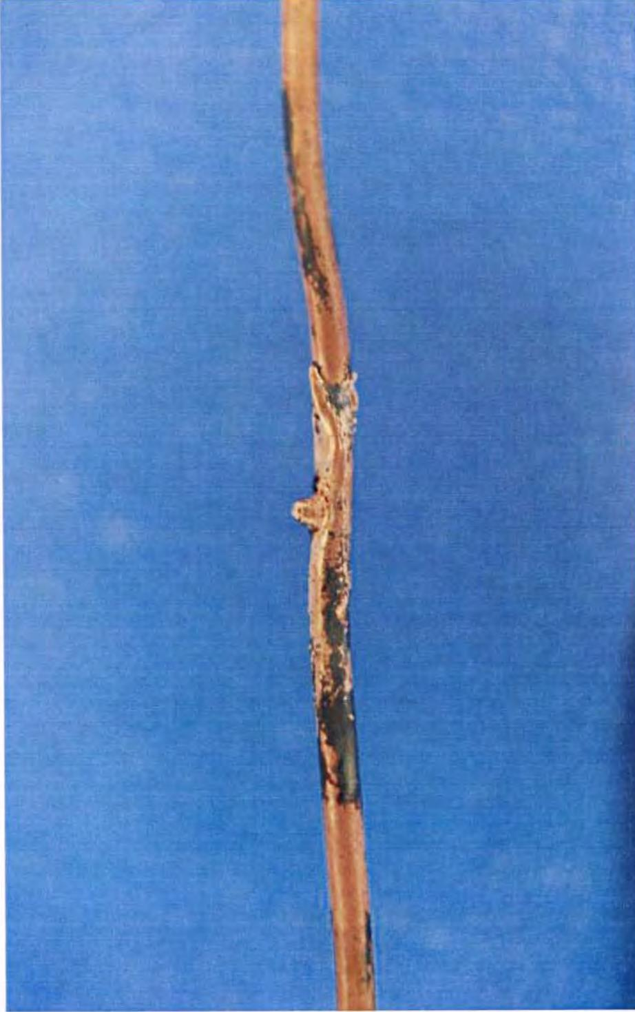
Photograph 18: Close-up view of the region identified in this supplemental report as 'B' captured during my recent visual examination of the fire alarm conductors (item #5). This artifact was positioned in the middle area of the conductor marked with ends 18 (southern extent) and 39 (northern extent) during the September 27, 2012, inspection by others. My measurements indicated this artifact positioned about 67 inches north of the field cut end near the roof ridge.
